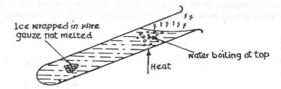
The diagram above illustrates the set-up for an experiment on heat conduction. The experiment demonstrates that
