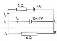
Using Kirchhoff's first law for electrical circuits, the current in the 6  $\Omega$  resistor in the diagram above will be
