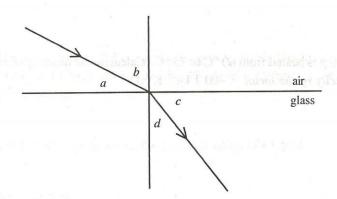
In the diagram above, the refractive index of glass relative to air is
